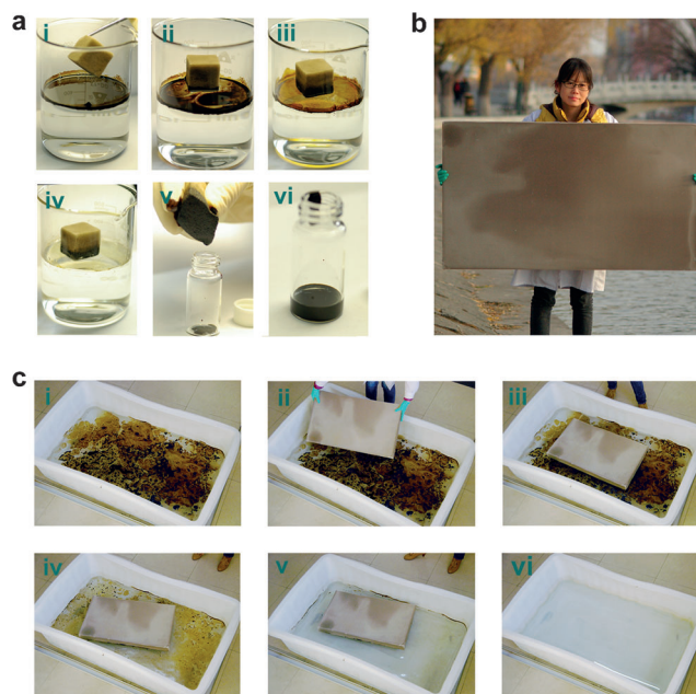
Figure 5. a) The absorption and recycling process of crude oil. b) The scalable manufacture of the superhydrophobic MF sponge (size: 120\text{ cm} \times 70\text{ cm} \times 5\text{ cm} ). c) Removal of crude oil from water using the superhydrophobic MF sponge (size of sponge: 70\text{ cm} \times 40\text{ cm} \times 5\text{ cm} ).
